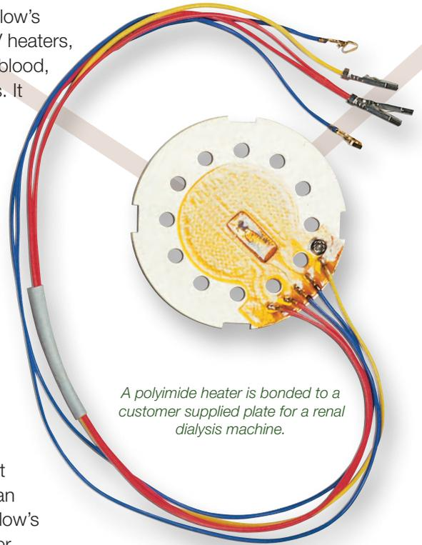
*A polyimide heater is bonded to a customer supplied plate for a renal dialysis machine.*
