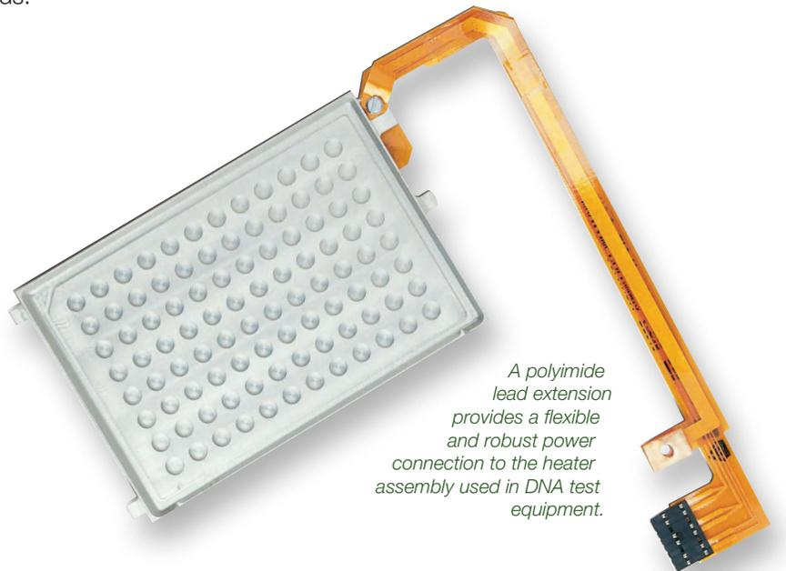
*A polyimide lead extension provides a flexible and robust power connection to the heater assembly used in DNA test equipment.*
