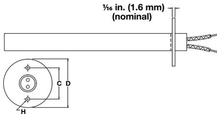
Stainless steel flanges are a convenient mounting method to position a heater within an application. The flange is staked on and located  $\frac{1}{4}$  in. (6 mm) from the lead end. The flange can be located up to  $2\frac{1}{4}$  in. (57 mm) from the lead end if it is over a no-heat section. Use this option in combination with most LA configurations.
