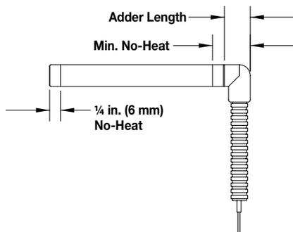
A right angle stainless steel hose is provided for wiring convenience. It protects leads from abrasion against sharp edges.
