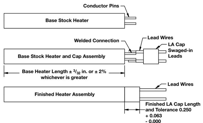
**Note:** Base stock heater tolerance + LA cap tolerance = total tolerance for assembly
