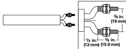
Post terminals provide a quick, secure connection with ring or fork connectors or bus bars. Threaded 6-32 studs are soldered to the solid power pins. Nuts and washers are provided.
