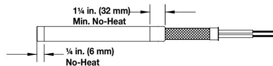
A straight stainless braid is designed to protect leads from abrasion against sharp edges and is Watlow's most flexible protective lead arrangement.
