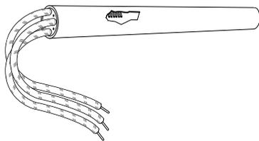
Ground leads are a safety feature to protect both workers and equipment. This configuration is not available on all options. Contact your Watlow representative for additional information. To order, specify **ground lead**.
