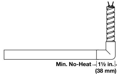
An LA right angle stainless steel hose with PTFE leads and a seal is the ultimate combination for providing abrasion protection and a moisture resistant seal with wiring convenience. Unless specified, a 12 in. (305 mm) hose is supplied. Leads are 2 in. (51 mm) longer than the hose but longer leads are available. This seal is effective to 392°F (200°C) under continuous operation.
