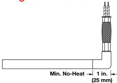
An LA right angle stainless steel braid is provided for wiring convenience. It protects leads from abrasion against sharp edges.
