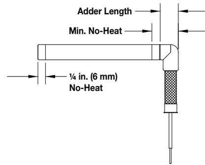
A right angle stainless steel braid is provided for wiring convenience. It protects leads from abrasion against sharp edges.
