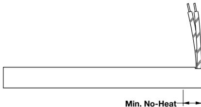
Right angle leads are used in applications with a high degree of flexing and when space limitations are critical. Lead wires exit at a 90° angle through the side of the heater sheath. Right angle tube may be necessary on certain constructions. To order, specify **right angle leads** and lead length.
