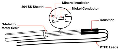
MI leads handle both high temperatures and contamination, and resist other problems including abrasion and excessive vibration. The metal seal and swaged-in formable MI cable leads can handle temperatures up to 1500°F (815°C). The lead end seal resists moisture and other forms of contamination, including gases, oils, plastic drool, solvents and water.
