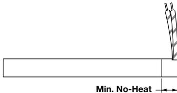
LA right angle leads are used in applications with a high degree of flexing and when space limitations are critical. Stranded lead wires are connected internally (swaged-in) and exit at a 90 degree angle at the end of the heater.
