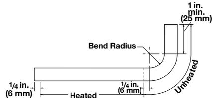
In applications where leads must exit at an angle, a bend can be made in the unheated section only. Heated sections may be on either side of the bend. It is recommended that the heater be bent at the Watlow factory.
