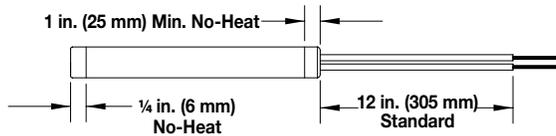
Swaged-in flexible leads are used in applications where a high degree of flexing exists or leads must be bent sharply adjacent to the heater without exposing or breaking the conductor. Stranded wire leads are connected internally and exit through the lead end.
