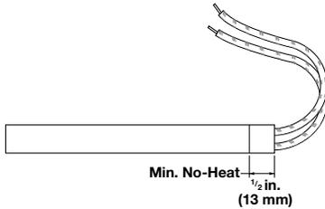
LA swaged-in flexible leads are used in applications where a high degree of flexing exists or the leads must be bent sharply adjacent to the heater without exposing or breaking the conductor. The stranded wire leads are connected internally and exit through the lead end. The overall length of the heater is extended by  $\frac{1}{4}$  in. (6 mm). To order, specify **length adder code E** bringing the total lead end no-heat to  $\frac{1}{2}$  in. (13 mm).
