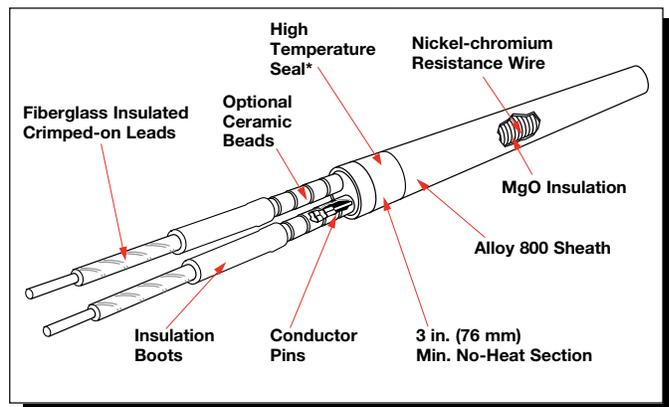
\* First 2 in. (51 mm) at lead end must be kept below 1000°F (538°C).
