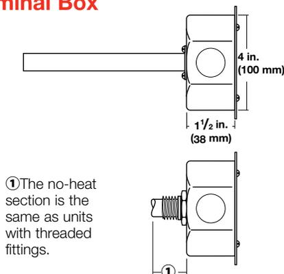
A 4 in. (100 mm) NEMA 1 octagonal terminal box is mounted on a flange or a threaded fitting. Boxes have  $\frac{1}{2}$  in. (13 mm) conduit knockouts for electrical connection. Hazardous location (NEMA 4 and NEMA 7) terminal boxes are also available. Contact your Watlow representative for details. Terminal boxes are available on  $\frac{1}{2}$  in. (13 mm) through 1 in. (25 mm) diameter FIREROD heaters. To order, specify **terminal box** and **NEMA type**.
