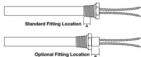
**Fitting overlaps the unheated section and is silver soldered to the sheath.**
