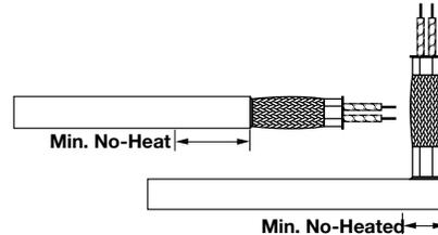
A stainless steel braid is designed to protect leads from abrasion against sharp edges. It is the most flexible of Watlow's protective lead arrangements.
