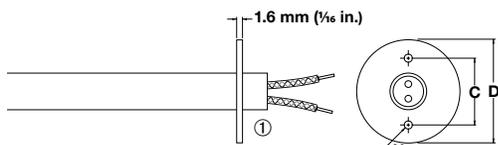
Stainless steel flanges are a convenient mounting method as well as a way to position a heater within an application. These flanges can be located in any no-heat section of the heater sheath. To order, specify **flange**, flange size and location.
