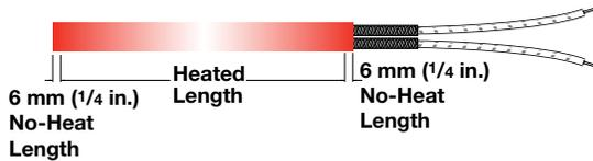
Distributed wattage varies the watt density along the length of the heater. This construction technique is used to compensate for heat losses along the edges of heated parts. To order, specify **distributed wattage** and give the length and wattage for each section.
