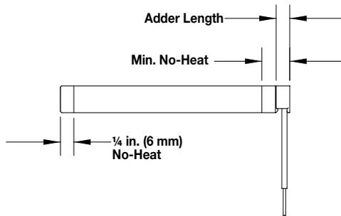
Right angle leads are used in applications with a high degree of flexing and when space limitations are critical. Standard lead wires are connected internally (swaged-in) and exit at a 90° angle at the end of the heater.
