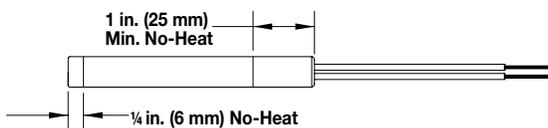
A PTFE seal and leads protect the heater against moisture and contamination from cleaning solvents, plastic material, fumes and organic tapes. This seal is effective up to 392°F (200°C) under continuous operation.
