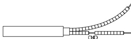
Ceramic bead insulation protects the leads from high ambient temperatures above 842°F (450°C).
