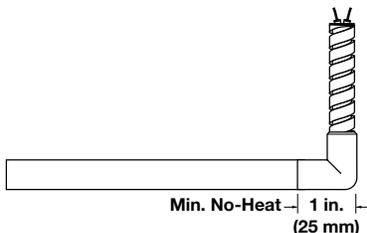
An LA right angle stainless steel hose is provided for wiring convenience. Like the LA straight stainless steel hose, it protects leads from abrasion against sharp edges. Unless specified, a 12 in. (305 mm) hose is supplied. Leads are 2 in. (51 mm) longer than the hose, but longer leads are available.
