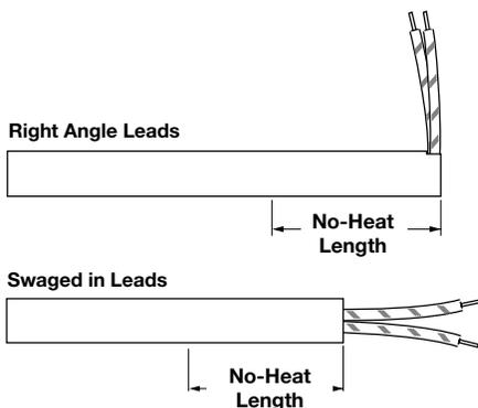
No-heat sections are recommended in applications where leads may be exposed to excessive heat, thus requiring a cooler lead end. Also use when heat is not required along the entire length of the metric FIREROD. No-heat extensions are available on all diameters with both pin style and swaged-in leads. To order, specify **no-heat** section and length of no-heat.
