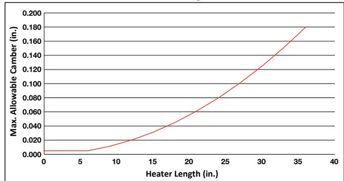
Max. camber = 0.020 in. x (length in feet)<sup>2</sup> or 0.005 in., whichever is greater.
