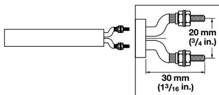
Post terminals provide a quick, secure connection with ring or fork connectors or bus bars. Threaded M4 x 12 mm studs are soldered to the solid power pins. Nuts and washers are provided. This termination is available on 16 and 20 mm (0.63 and 0.79 in.) diameter units. To order, specify **post terminals**.
