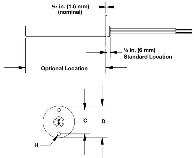
Stainless steel flanges are a convenient mounting method and can be used to position a heater within an application. The standard location is 1/4 in. (6 mm) from the lead end. However, a specific location may be requested in any location along the no-heat section. Unless specified, flanges are staked to the sheath.
