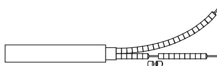
Ceramic bead insulation protects the leads from high temperature ambients above 450°C (840°F). The beads fit over solid conductors and are extended long enough to reach a cooler area where flexible wires can be attached. To order, specify **ceramic beads** and length, and additional lead length.
