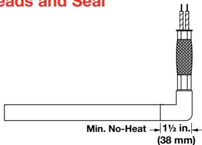
The LA right angle stainless steel braid with PTFE leads and seal is Watlow's most flexible lead protection with a moisture resistant PTFE seal and wiring convenience. Unless specified, a 12 in. (305 mm) braid is supplied. Leads are 2 in. (51 mm) longer than the braid, but longer leads are available. This seal is effective up to 392°F (200°C) under continuous operation.
