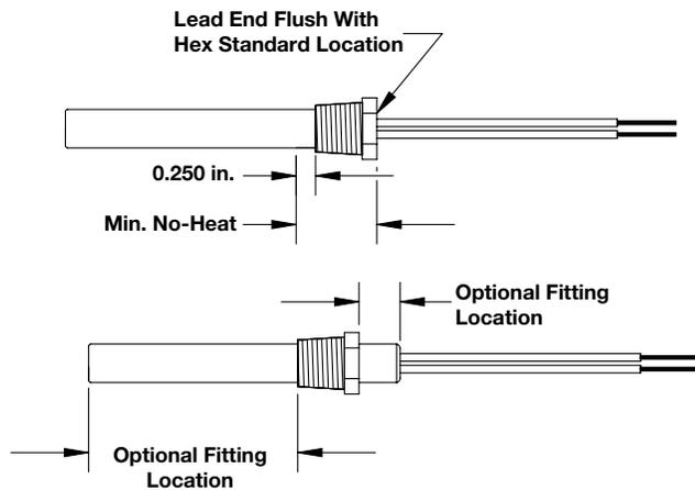
Threaded fittings allow fast, water-tight heater installation into a threaded hole. Standard fittings are 304 stainless steel and welded to the heater sheath. Other materials are available upon request. Double threaded fittings are also available.
