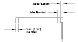
Right angle leads are used in applications with a high degree of flexing and when space limitations are critical. Standard lead wires are connected internally (swaged-in) and exit at a 90° angle at the end of the heater.
