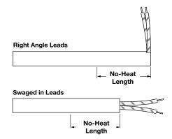
No-heat sections are recommended in applications where leads may be exposed to excessive heat, thus requiring a cooler lead end. Also use when heat is not required along the entire length of the metric FIREROD. No-heat extensions are available on all diameters with both pin style and swaged-in leads. To order, specify **no-heat** section and length of no-heat.
