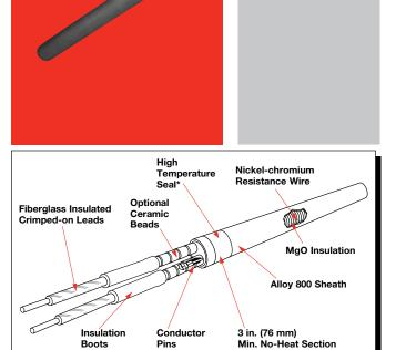
\* First 2 in. (51 mm) at lead end must be kept below 1000°F (538°C).
