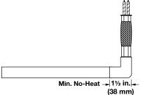
The LA right angle stainless steel braid with PTFE leads and seal is Watlow's most flexible lead protection with a moisture resistant PTFE seal and wiring convenience. Unless specified, a 12 in. (305 mm) braid is supplied. Leads are 2 in. (51 mm) longer than the braid, but longer leads are available. This seal is effective up to 392°F (200°C) under continuous operation.
