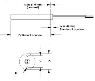
Stainless steel flanges are a convenient mounting method and can be used to position a heater within an application. The standard location is <sup>1</sup>/4 in. (6 mm) from the lead end. However, a specific location may be requested in any location along the no-heat section. Unless specified, flanges are staked to the sheath. To order, specify **flange size** and location.
