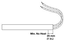
Swaged-in flexible leads, with silicone-fiberglass insulation, are recommended for applications in which the leads must be bent at the exit point from the heater. Unless longer length is specified, 250 mm (10 in.) leads are supplied.
