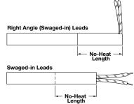
No-heat extensions are recommended in applications where leads may be exposed to excessive heat and require a cooler lead end. They are also used when heat is not required along the entire length of the FIREROD.
