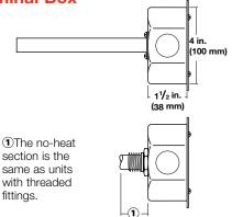
A 4 in. (100 mm) NEMA 1 octagonal terminal box is mounted on a flange or a threaded fitting. Boxes have <sup>1</sup>/<sub>2</sub> in. (13 mm) conduit knockouts for electrical connection.
