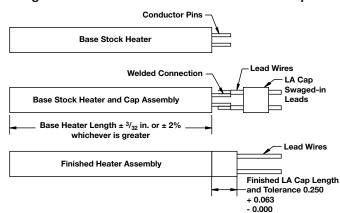
Note: Base stock heater tolerance + LA cap tolerance = total tolerance for assembly
