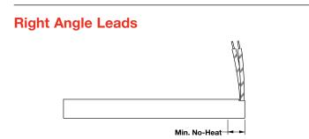
Right angle leads are used in applications with a high degree of flexing and when space limitations are critical. Lead wires exit at a 90° angle through the side of the heater sheath. Right angle tube may be necessary on certain constructions. To order, specify **right angle leads** and lead length.
