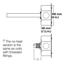
NEMA 1, NEMA 4 (moisture-proof) and NEMA 7 (explosion-proof) octagonal terminal boxes can be mounted to a flange or threaded fitting on the 12.5, 16 and 20 mm diameter units. These 100 mm (4 in.) terminal boxes have conduit knockouts to protect electrical connections.
