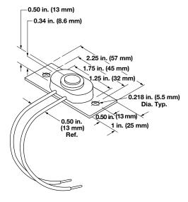
**Note:** For direct control of air temperature as is required in enclosure heating applications, specify thermostat model number ST-207E. This is a modified ST-207 mounted on <sup>1</sup>/<sub>32</sub> inch thick G-10 circuit board with the thermostat's metal cap exposed to sense air temperature.
