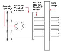
Stand-off terminal enclosures provide an air-insulating barrier between the flange and terminal enclosure by mounting the terminations and wiring away from the flange. Stand-off terminal enclosures are recommended whenever a process operating temperature exceeds 210°F (100°C). This helps minimize terminal enclosure temperatures.
