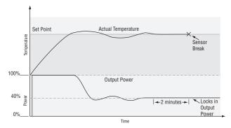
Input Error Latching  $\car{Ler}$  (Setup Page, Analog Input Menu) determines the controller's response once a valid input signal returns to the controller. If latching is on, then the controller will continue to indicate an input error until the error is cleared. To clear a latched alarm, press the Advance Key () then the Up Key ().
