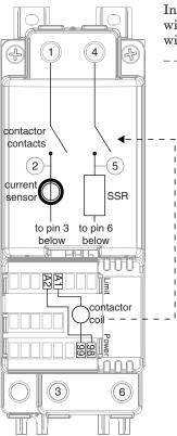
Internal wiring in an ST with a double-pole contactor without a limit (ST  $\_$  B - F  $\_$
