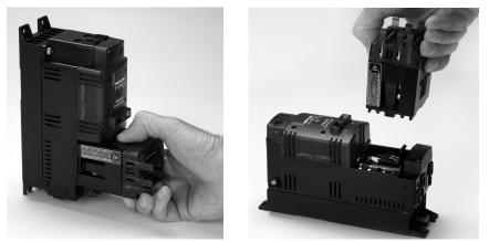
1. Pinch the release levers on the top and bottom of the control module and lift the right edge forward to detach the unit.
