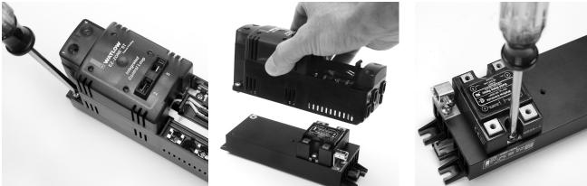
3. With a Phillips screwdriver, remove the two screws at the top corners of the controller.
