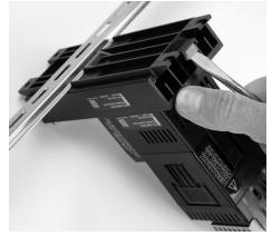
To dismount the controller, first use a screwdriver to pull down the small lever on the bottom of the heat sink and rotate the bottom of the controller forward. Then lift the the controller off of the rail.
