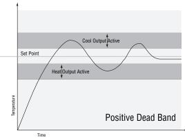
When the **dead band value is zero**, the heating output activates when the temperature drops below the set point, and the cooling output switches on when the temperature exceeds the set point.
