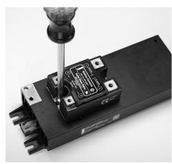
4. Using a Phillips screwdriver, remove the two screws connecting the solid-state relay to the heat sink.
