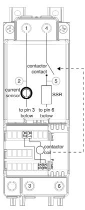
Internal wiring in an ST with a single-pole contactor without a limit (ST  $\_$  B - B  $\_$
