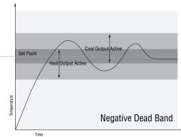
Adjust the dead band with Dead Band \_\_\_\_\_ (Operations Page, Loop Menu).
