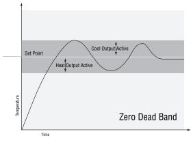
When the **dead band value is a negative value**, both heating and cooling outputs are active when the temperature is near the set point.
