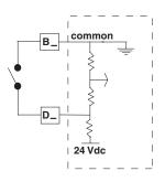
NOTE: To prevent ground loops, isolation needs to be maintained from input to output when using switched DC or analog process outputs.
