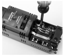
2. With a Phillips screwdriver, remove the four nearest screws that were under the module.
