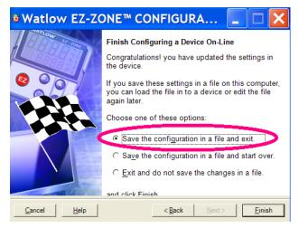
Although the ST control now contains the configuration (because the previous discussion focused on doing the configuration on-line) it is suggested that after the configuration process is completed that the user save this file on the PC for future use. If for some reason someone inadvertently changed a setting without understanding the impact it would be easy and perhaps faster to download a saved configuration back to the control versus trying to figure out what was changed.
