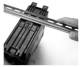
To mount the controller on a DIN rail, first hook the top flange on the back of the heat sink on to the top of the DIN rail. Then rotate the controller to an upright position until the lower flange snaps into place.
