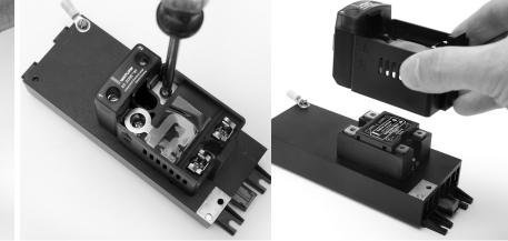
2. With a Phillips screwdriver, remove 3. Lift the controller body, exposing the four nearest screws that were un- the solid-state relay. der the module.
