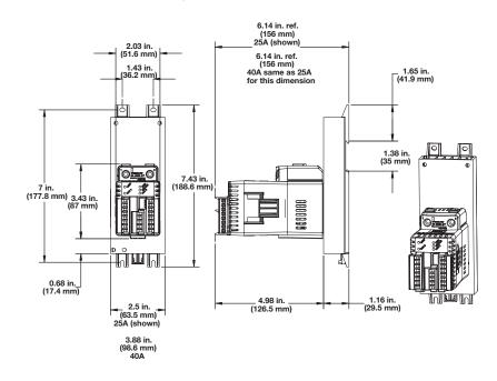
**Note:** EZ-ZONE ST must be mounted vertically (as shown) to meet amp/ambient performance curve.
