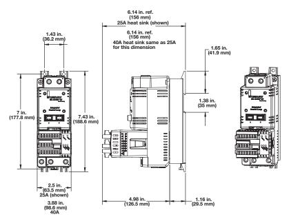
**Note:** EZ-ZONE ST must be mounted vertically (as shown) to meet amp/ambient performance curve.
