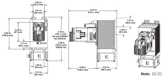
**Note:** EZ-ZONE ST must be mounted vertically (as shown) to meet amp/ambient performance curve.
