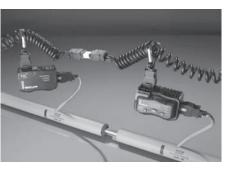
The EHG SL10 can be "daisy-chained" for gas line and other assemblies.
