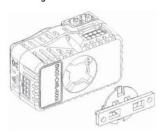
The Series EHG SL10 mounting bracket lets you mount the controller in any of four angles. After disconnecting both wiring connectors, gently rotate the controller counterclockwise until it unlocks from the mounting bracket. Re-orient the controller on the mounting bracket and gently rotate it clockwise until it locks.
