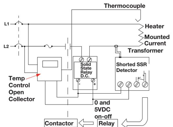
**Note:** Semiconductor power switching devices are not legal for over temperature limit or safety devices. For limit and safety devices you must have a positive mechanical break of all electrically hot legs simultaneously.
