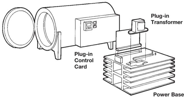
In heat treating applications, the QPAC offers modular flexibility. Different heater elements require different control firing modes, for example, tungsten elements need phase-angle firing, while Nichrome® elements use burst (zero cross) firing.
