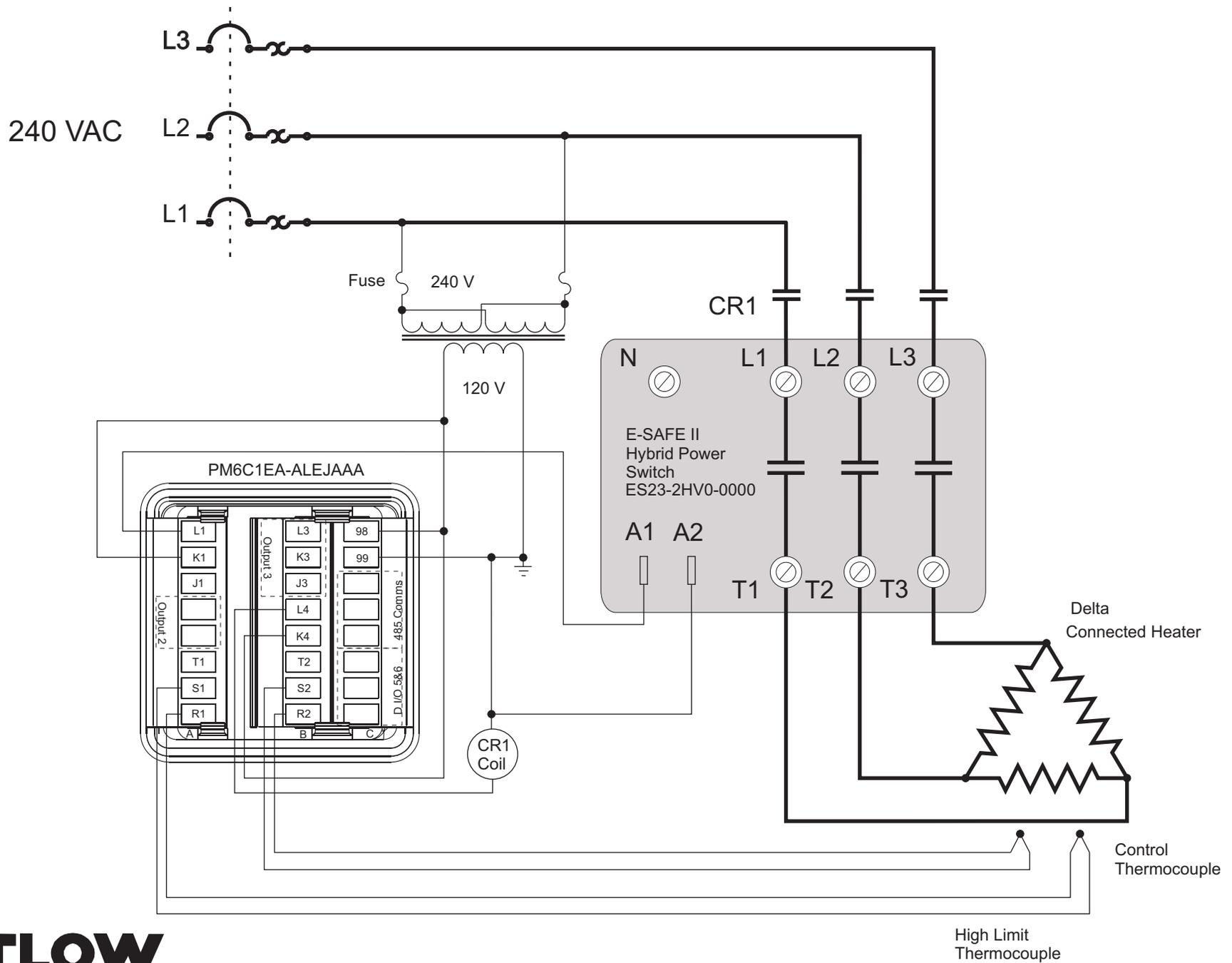
ESAFE II System Wiring Example
