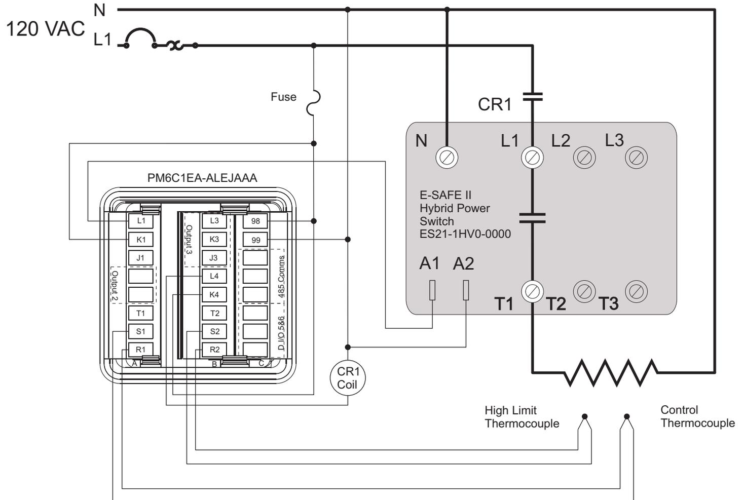
ESAFE II System Wiring Example
