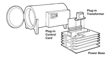
In heat treating applications, the QPAC offers modular flexibility. Different heater elements require different control firing modes, for example, tungsten elements need phase-angle firing, while Nichrome<sup>®</sup> elements use burst (zero cross) firing.
