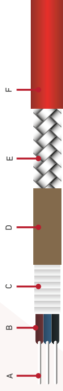
A. Tinned Copper Stranded Wire B. FEP Insulation Layer C. Ni-Cr Alloy Wire D. PEP Insulation Layer E. Tinned Copper Metal Braid F. Outer Jacket
