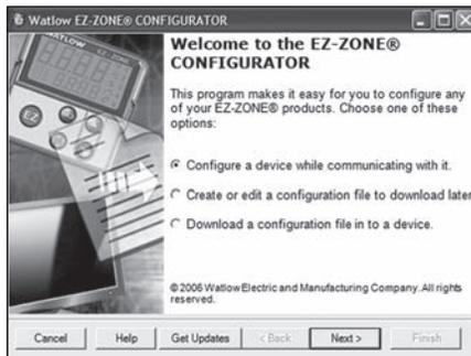
The EZ-ZONE configurator software is used to set up Watlow EZ-ZONE products in one simple process. It works without requiring the purchase of any communication options because it uses the standard bus communications protocol that is included with all EZ-ZONE products. EZ-ZONE configurator can be used for online and offline configurations and downloading previously saved setups. It is available as a FREE download at [www.watlow.com](http://www.watlow.com). See page 397.
