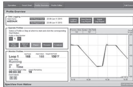
SpecView is designed for industrial users and includes features such as data logging, trending and support for bar code readers and touch screens. Errors are reduced for any process by creating application-specific screens. The software provides a historical replay option, easy-to-use recipe features and remote access options, including LAN, Internet and modem. See page 385.
