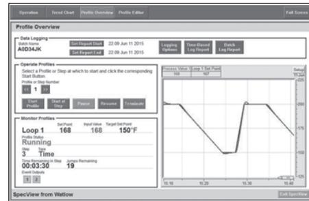
SpecView is designed for industrial users and includes features such as data logging, trending and support for bar code readers and touch screens. Errors are reduced for any process by creating application-specific screens. The software provides a historical replay option, easy-to-use recipe features and remote access options, including LAN, Internet and modem. See page 385.
