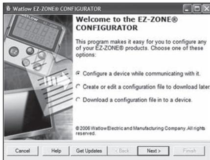
The EZ-ZONE configurator software is used to set up Watlow EZ-ZONE products in one simple process. It works without requiring the purchase of any communication options because it uses the standard bus communications protocol that is included with all EZ-ZONE products. EZ-ZONE configurator can be used for online and offline configurations and downloading previously saved setups. It is available as a FREE download at [www.watlow.com](http://www.watlow.com). See page 397.
