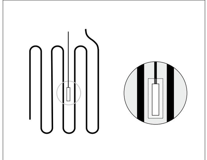
After completing installation of the heating tape this is glued over with aluminium self-adhesive tape or the tank is wrapped in aluminium foil.
