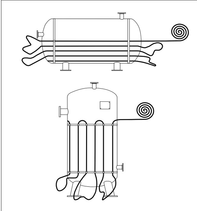
After installing the heating tape, this is then aligned exactly according to the project planning specifications and fixed firmly to the bases and the cylinder using the clamping rings provided. In doing so care should be taken that the clamping rings are not tightened too firmly so as not to damage the heating tape. It should be possible to move the heating tape slightly under the clamping ring.
